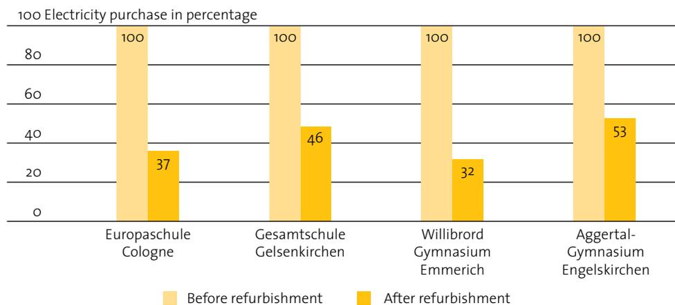
Figure 7: The electricity purchase at the four Solar&Spar schools was significantly reduced
